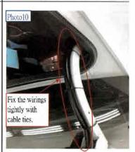
12.Use the cable ties to fix the wirings onto t truck bracket.
