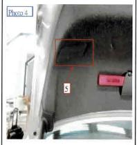
5. Remove the trim panel of the inner lamp.
