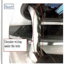
Step2-4: Arrange the wirings.
