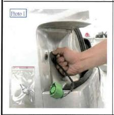
1. Remove the trim panels of the rear lamps and remove the genuine lamps.
