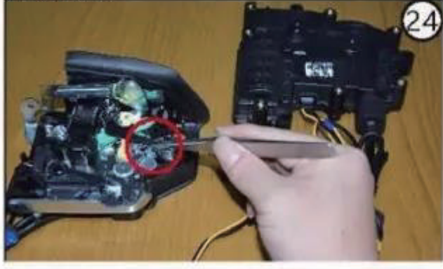
5. Before assembling the electric lock and the central control unit, please lay out and fix the L-type transmission arm on the electric lock, so as to facilitate the next step of installation (FIG. 24).
