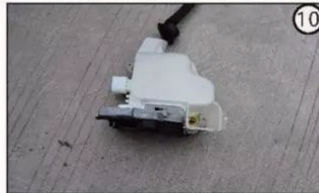
10. Remove the door lock of the original car and put it in good condition (figure 10)
