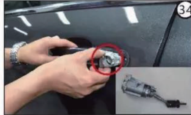
2. Install the assembled electric lock back to the original lock position and restore the key to enter the lock core (figure 33)
