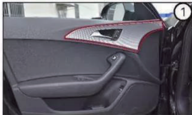
1. Decorate panel with skid plate wei to open internal door handle (figure 1)
