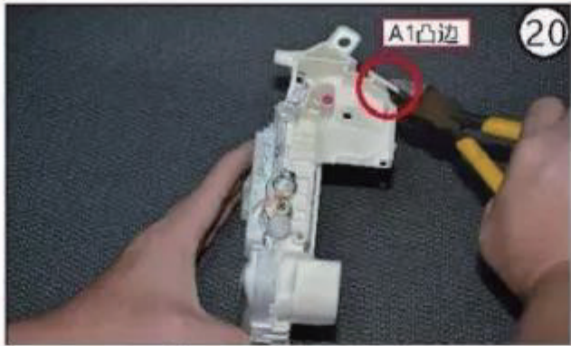
1. Trim the A1 convex edge on the shell of the central control unit of the original door lock with pliers (please refer to the limited height supervision of Mafoping for the A1 convex edge in fig. 22) (fig. 20)
