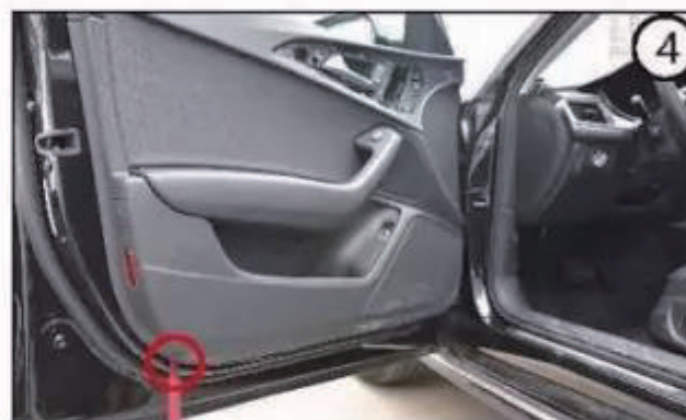
4. Use the skid plate to carefully pry the fastener around the interior door decoration plate of the driving door (note: check whether all the fixed screws on the interior door decoration plate are removed before prying) (figure 4)
