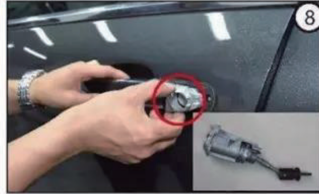
8. Pry the key on the main driving door with a skid plate to enter the decorative cover plate of the lock core and take out the lock core (figure 8)
