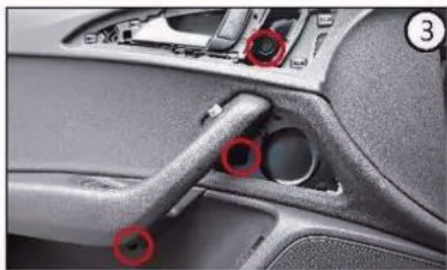
3. Three fixing screws for interior door trim plate in the unloading process (FIG. 3)
