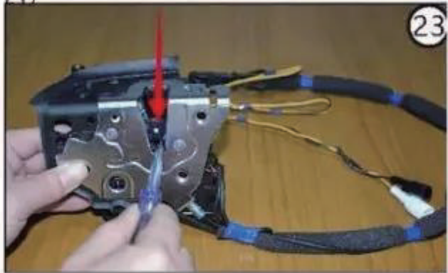
4. Use a circular bar with a diameter of 500mm to press the lock tongue on the electric suction door lock to the full lock position (this step pays special attention to prevent the door detection switch from being crushed when the lock core and the central lock control unit are assembled) (figure 23)
