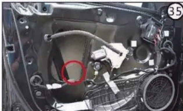
3. Place the motor box on the sheet metal reinforcement inside the door. Joint position need to choose the plane, the motor box below the power cord should be along the door leads to the outer, the diaphragm to straighten out the wiring harness and rolling with fixed light according to the control of glass falling slowly, the watch glass with the motor box and electric Cong harness if there is interference, if no interference phenomenon, with a marker pen marking (figure 34)
