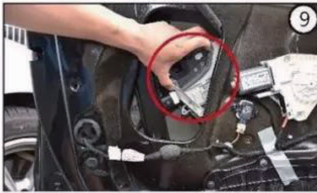
9. Carefully remove the original door lock from the side of the inner door (FIG. 9)
