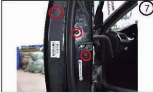
7. Open the front left door side key to enter the lock core screw rubber waste, remove the lock lock screw (figure 7)
