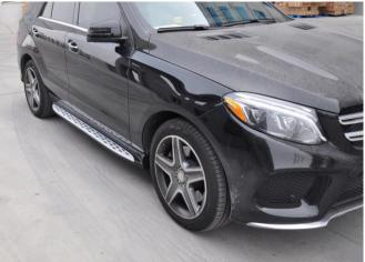
5. INSTALLATION FINISHED, CHECK CAREFULLY IF THE RUNNING BAORD APPRESS THE BODY, IF NOT, PLEASE MAKE SURE ALL PARTS ARE INSTALLED CORRECTLY.
