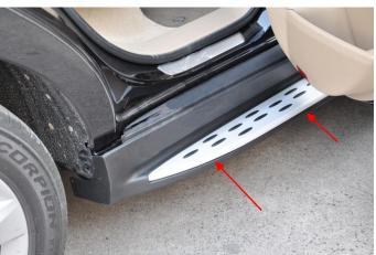
4.PUT SIDE STEPS ON, AND PUSH IT TO MAKE IT TIGHTLY WITH THE BODY, THEN INSERT EXPANSION
