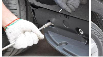
3. ADJUST SIDE STEPS SUPPORT TO MAKE IT ALIGN WITH CAR BODY, AND TIGHTEN ALL SCREWS.
