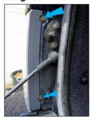
Be careful not to mark the paint or crack the lens. If the bottom fitting is tight try the top fitting etc.
