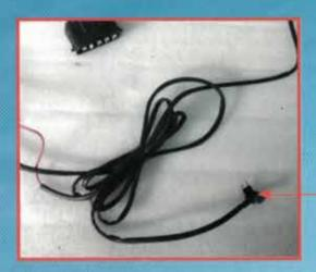
OPEN THE FRONT DRIVER SIDE FUSE BOX, ACC WIRE CONNECT WITH THE APPROVEDOR
