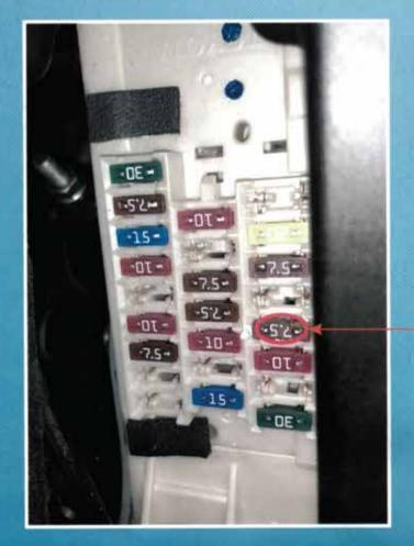
OPEN THE FUSE BOX UNDER THE STEERING WHEEL OF THE CAB. PLUG OUT THE 7.5A FUSE. REMOVE APS ERROR CODE
