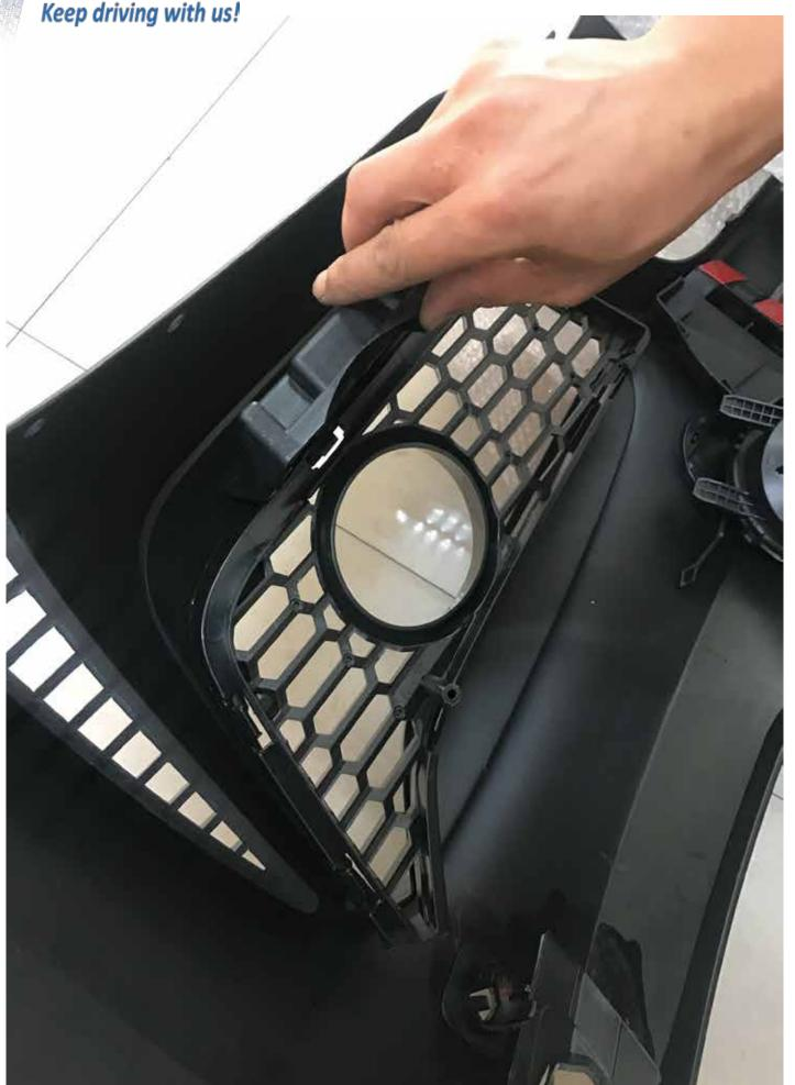
Step 3: Fix the projector to the bar with the screws
