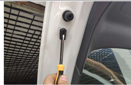
9. Pry open the gas spring snap ring and remove the pole of the original car (same left and right)
