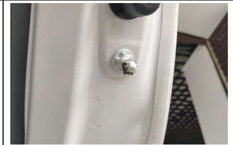
10. Remove the original tailgate screw ball (same left and right)
