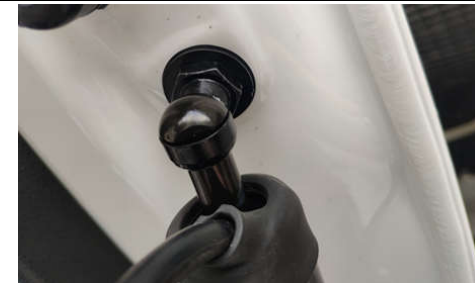
11. Install our screw ball and gasket (same left and right)
