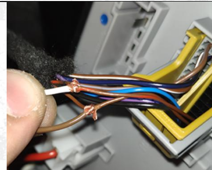
21. Our white line is connected to the original reddish brown line (CAN-H) Our brown line is connected to the original pure brown line (CAN-L)
