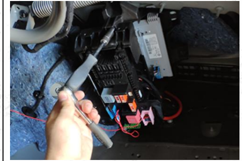
20. Move the fuse box for find the can line.
