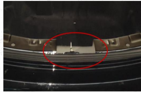
14. Assemble lower lock ring back, and screw stable on the car with M6 screws.
