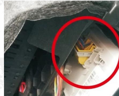
19. Find the Yellow plug behind the fuse box, Can line in this place.
