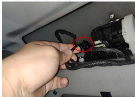
17. Pull out original rear switch joints And then contact with our wire harness
