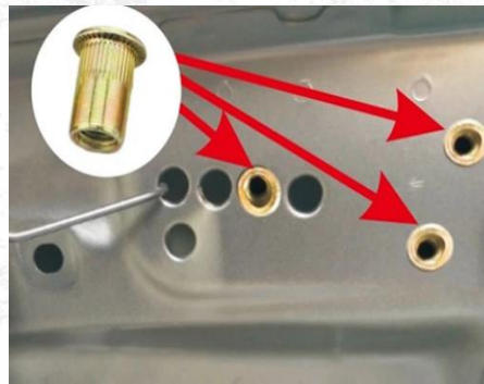
4. Mount three M8 rivets on both sides of rear trunk. As pictures shown.
