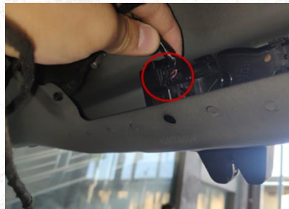
16. Pull out original lock signal joints And then contact with our wire harness.
