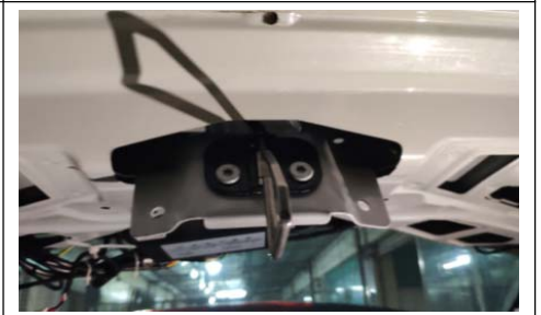
12. Install the lock of our company (use the original screw and the nut provided by our company)
