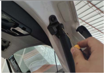
3. Pry off the original car gas spring retainer and remove the pole (same left and right)
