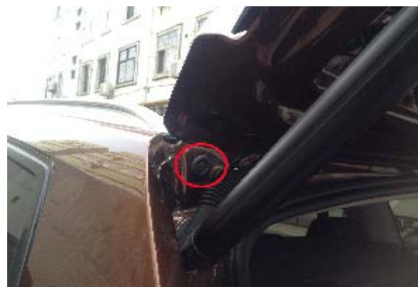
5. Pull out the reserved rubber plug of the original car (same left and right)
