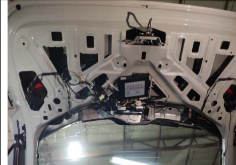
21. Connect the control box harness and fix the control box
