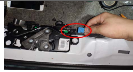
7. Pull out the original car lock cable and dock with our cable
