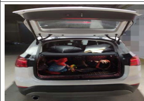
22. Recover all trims, and close the door once after installation, so as to initialize the system
