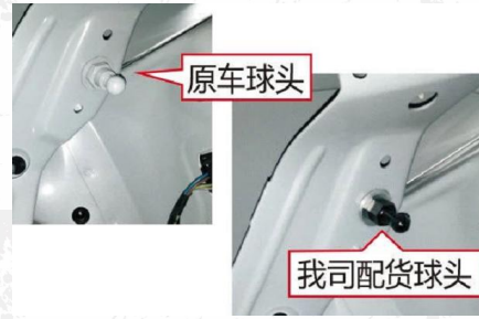
7. Installation of ball head provided by our company (same left and right)
