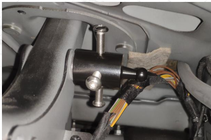
5. Put the ball head sleeve of our company into the ball head of the original vehicle, and lock the M6 screw (same left and right)
