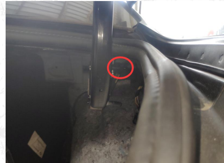
4. Find the ball head of the original car on the swing arm (same left and right)
