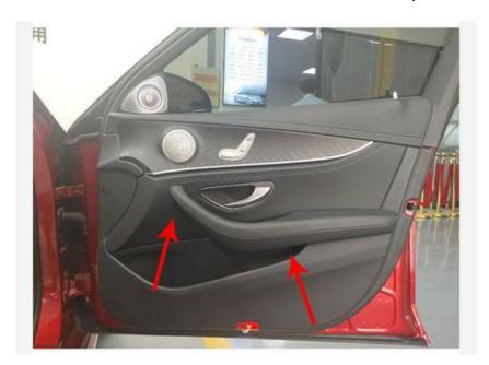
2. Use two long flat blade screwdrivers to pry up and down to remove the small wooden frame.
