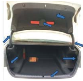
2. Remove the tailgate trim in turn
