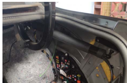
6. Install our electric pole ("L" left, "R" right)
