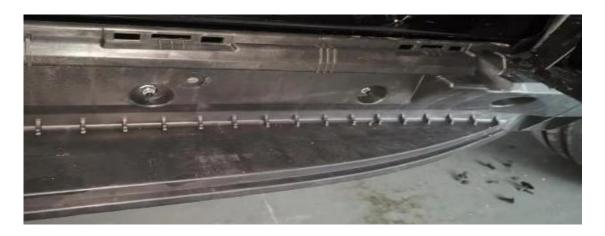
3. Align the pedals with the holes in the frame and install them on the frame, and pat tightly (tighten the bottom first, then the upper part)
