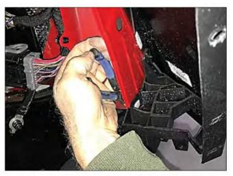
Disconnect the light wire harness (in the circle) by pushing the red tab out to unlock. Push in the release tab and pull the harness out. To remove lower bracket, use pliers behind bracket and sheet metal to disengage two white factory retainers and discard.
