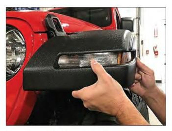
Holding the flare on the fender, install two supplied plastic retainers through the holes at bottom rear of flare, under flare corner bracket feature, and into holes in fender. Push each retainer in to engage. Fit assembled light housing bracket into inside of flare, as shown.
