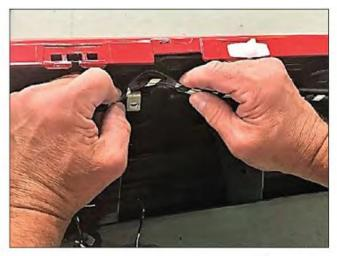
Lift the housing flap up to remove four more fasteners underneath it as shown using the T-30 Torx driver. Remove the wiring harness from light housing routing using your hands or pliers. Do not cut the electrical tape. Gently pry from contact points. Disconnect light bulb connector. Remove the light from the factory flare.
