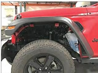
Install the seven remaining plastic fasteners. Repeat instructions to this point for the other side of the vehicle.
