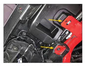
Using a 10mm socket, remove the three factory bolts from locations marked by arrows. Remove and discard wheel well liner. Remove two bolts from the light housing but retain those for use in Step 17.
