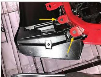
Using a 10mm socket, start two factory bolts (removed at Step 3) through sheet metal brackets and into t-nuts present on light housing bracket. Do not tighten.
