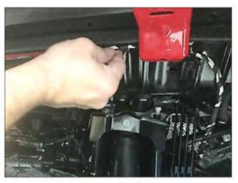
Route wiring harness from light housing over the first of the metal fender brackets and toward the channel molded into flare. Tuck wiring harness up into channel in flare and route into engine compartment (connector is located near washer fluid reservoir). Connect wiring harness to connector.
