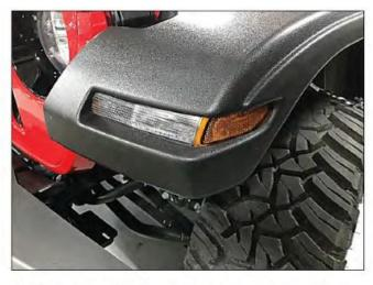
Using a Phillips screwdriver, start two supplied Truss screws through clip holes in the bracket and into the flare inner structure. Do not tighten. Check fit of light inside light pocket and adjust screws incrementally as needed to ensure even spacing between light and flare. Slowly tighten ALL screws and bolts in light housing and bracket. It is intentional that parts of the light lenses will be obscured by the flare.
