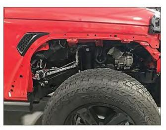
Disengage the nine white factory retainers that are holding the factory flare onto vehicle. These are spaced along the wheel well. All but one bracket is accessible by pliers. If you wish to preserve the paint finish (which will be covered by flare), use a plastic pry tool to help remove retainers. Pull factory flare from vehicle. Pry any white retainers from the sheet metal and discard. These holes must be clear for installation. Retain factory flare to remove light housing in the next steps.
