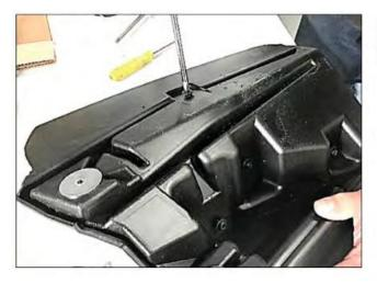
Start a supplied Truss screw into clip. Screws will not be tightened until after the light housing is installed in new flare.
