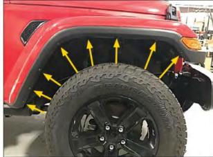
Put on safety glasses and gloves. On front factory flare, use an awl to pop the eight factory retainers in center of each retainer to disengage. Arrows point to the location of factory retainers.
