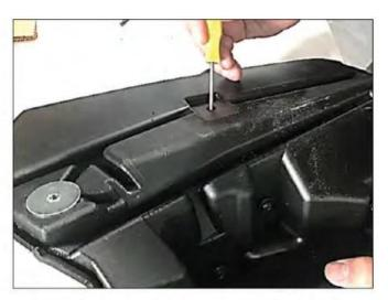
Assemble the modified light housing with supplied front bracket. Start three factory fasteners (removed at Step 6) through supplied Front Bracket and into modified light housing, but do not tighten. Using an awl, make sure "U" clip installed previously is still centered over hole in bracket.
