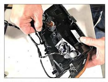
Install a supplied "U" Clip over hole in bottom bracket of modified light housing, centering the hole in clip over the hole in the bracket. Reconnect harness and/or light bulbs if you removed them. The wire harness will need to be routed in the groove in the housing and ultimately to the connector in the engine compartment when installing new flares.
