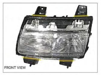
Using a cutoff wheel or saw, cut the four plastic tabs on light housing as shown. The yellow line denotes the locations to cut. The goal is to remove these tabs parallel with contours of light housing as cleanly as possible. Take precaustions to avoid cutting away too much material from light housing. Use the next pictures to help visualize where to make cuts. Do not cut into the sealed clear lens or housing.
