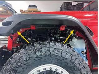
Slide the two supplied "U" clips onto the front flare inner bracket as shown. Holding the flare on the fender, install two supplied plastic retainers through the flare holes located at the arrows. Push each retainer in to engage. The remaining plastic retainers will be installed in later steps.
