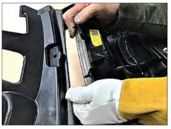
Slide the side marker light from the housing. Light is taped to the factory flare. Gently pry the housing from flare to disengage tape.
