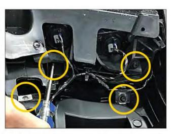
Turn the removed flare on its back on a work surface. Using a Phillips screwdriver, remove the factory fastener from the light housing as shown. Using a T-30 Torx driver, remove the four factory fasteners as shown. Retain ALL factory fasteners as most will be reused in Steps 9 and 13.
