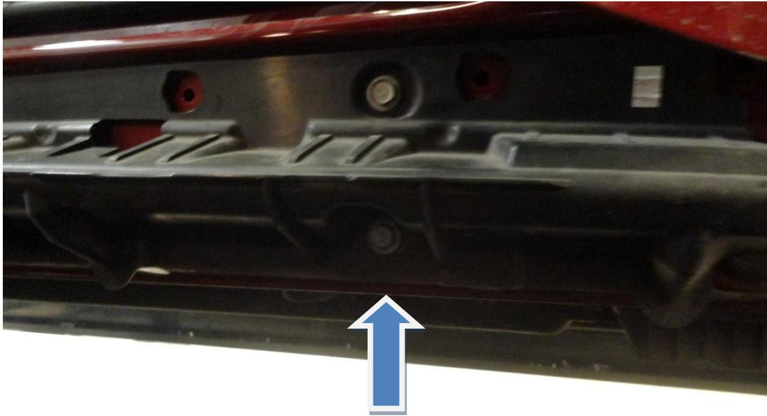
**Step 4:** Install the clips on the pointed position
